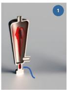
A jet of high pressure air is shot through the powder chamber, aerosolising the powder upwards into the holding chamber. The energy of the jet is siphoned off.
