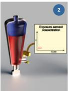
The aerosol rises upwards in a plume, then settling downwards in the holding chamber where a controlled air flow "pulls" the API past a real-time aerosol monitor.
